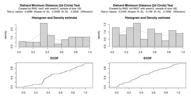
Figure 1: Comparison of ran0 and mt19937 under test 2dsphere
